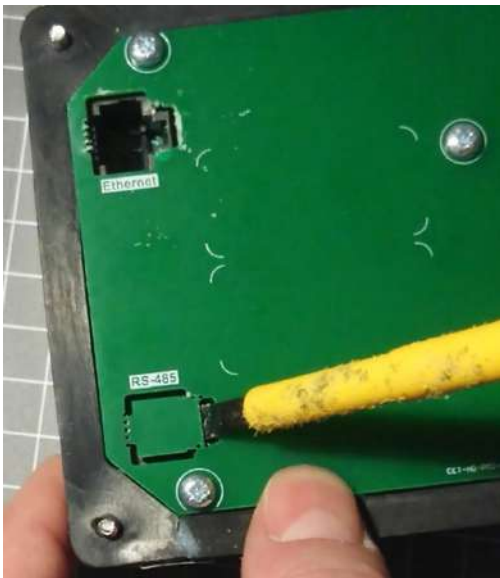
RS485 Port on CET-HD-PM2-1 Power Meter
